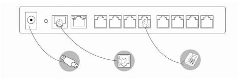
Figure 3-1 TA800 Connection Diagram
