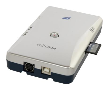
The V-Tap ISDN BRI is a device that can record the calls from an ISDN-2 line.
